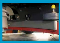
Easily remove the squeegee with the push of a button.
